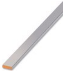
Neutral busbar, DIN VDE 0611-4: 1991-02, material: Copper, tin-plated, color: silver
